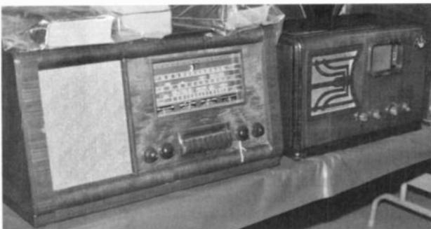
Two radios that use tuning eye tubes — the GE with push-button tuning a large "slide-rule" dial, left, sold for \$100; the Airline Model 62-318 "movie-dial," right, sold for \$45.
