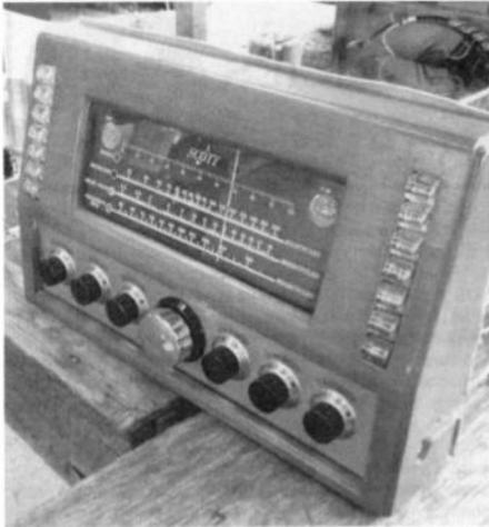
*This E.H. Scott Model 800B receiver, ca. 1946, with 24 tubes, was the last of the Scott radios.*
