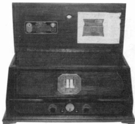
**RCA RADIOLA 25** – This 6-tube battery set was manufactured in 1925 by the Radio Corp. of America (RCA). It operates on five Type 199 tubes, and one Type 120 tube for output. It tunes with two thumbwheel dials in the brass escutcheon. The hole in the top lid is for a rotating loop antenna. (Clark Trissell – Lincoln, NE)
