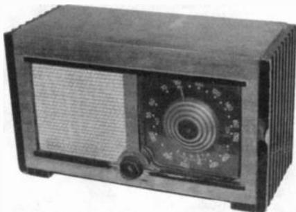
**ZENITH MODEL 5D027** – Manufactured in 1942, this 5-tube receiver has an AC/DC circuit and tunes the broadcast band only. Tubes used in the circuit are one each of the following types: 35Z5, 50L6, 12SQ7, 12SK7, and 12SA7. (Clark Trissell – Lincoln, NE)
