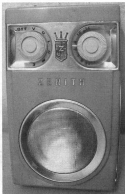
Figure 4. In 1957, Zenith switched from hand-wiring to printed circuit board construction on this 500B series with its white station indicator on the tuning knob collar.
