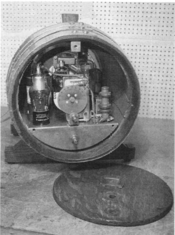
Figure 11. The restored radio showing how the radio chassis fits inside the keg.
