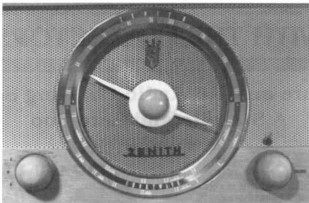
Figure 2. The markings across the top of the large dial are for the broadcast band. Along the bottom are the two shortwave bands. The right small knob is for volume; the left knob has two concentric knobs the outer is for tuning, the inner is the band switch.
