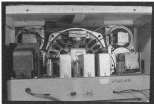
Figure 3. A rear inside view of the Zenith set. Note the two "tweeters" on each side of the larger main speaker. The text "Chassis 6Y61B" can be seen on the right/top of the chassis.
