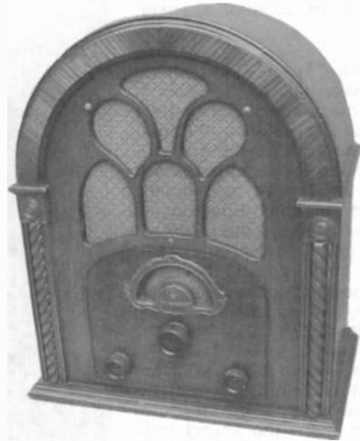
**ATWATER KENT MODEL 92** – This beautifully styled cathedral was manufactured by Atwater Kent in 1931. It has distinctive "rope-twist" trim on the front. An 8-tube Superheterodyne, it tunes the broadcast band only. (Dave Crocker – Mashpee, MA)
