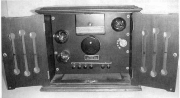
From Western Electric, a Model 14A amplifier/speaker with three Type VT-1 tubes sold for \$600. The horn and grille are on the other side.
