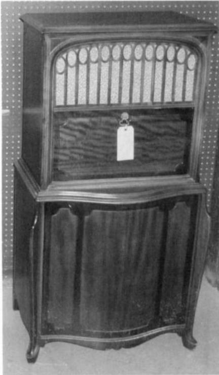
An RCA Radiola Super VIII, ca 1924, in its impressive cabinet. This battery-operated radio sold for \$200.
