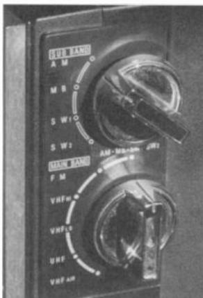
Figure 5. The side-mounted controls on the Patrolman 9.
