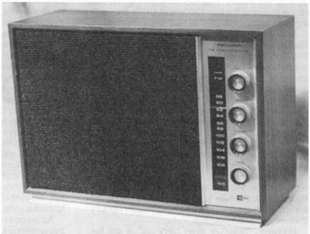
*Figure 1. The RadioShack Realistic FM Concertmaster was an early entry in the FM-only radio market.*
