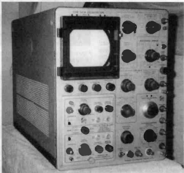
Figure 1. The Tektronix Type 545A scope as found with plug-ins and a camera bezel.
