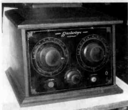
With its unassuming exterior, this Standardyne 2-dialer, is unusual inside. It is a multivalve set utilizing an early vacuum tube which contains three triodes. It sold for \$275 in the auction.
