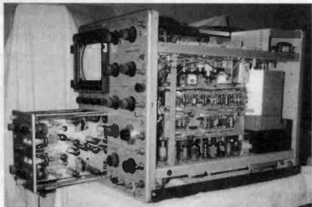
Figure 2. A right view of the Type 545A showing the Type CA dual trace plug-in to show its tubes. A dual-trace module allows two different signals to be displayed simultaneously, one above the other on the CRT face.
