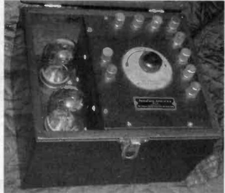
Seen in the flea market, this AeroFone 2-tube amplifier was manufactured by the Prometheus Electric Co., New York. It was designed to be used with the Aeriola Sr. receiver as shown below. The literature with the amplifier claimed that "... it will give results that are almost unbelievable. It will amplify the volume... to such an extent that a loud speaker can be operated."
