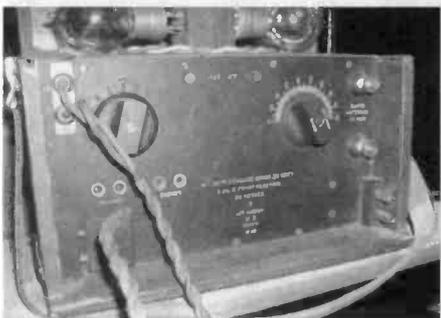
This wireless item from World War I is a British Mark II receiver used at the front. In its fabric-covered wood case, it utilizes two Type R valves as an oscillating detector and an AF amplifier. According to Jonathan Hill in "Radio Radio," it tunes 80 to 65 meters. In the auction, it sold for \$1,000.
