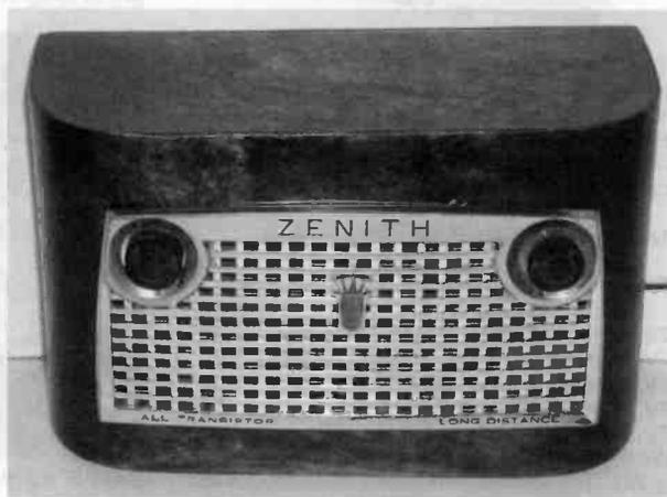
Figure 2. The Zenith Royal 750 in its new wood cabinet. The grille, a classic of its day, is made of diecast anodized aluminum.
