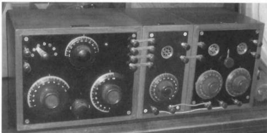
The three-panel "Cleveland Waves To You" set, shown above, sold for \$1,600. The panel functions are tuner, detector, and 2-step amplifier. An unusual item, this particular example was at one time in the Muchow collection. The nameplate, shown at right, is an artistic departure from the usual radio nameplate. The lettering superimposed over a wave-shaped line is: "wCaLvEEVsEtLoAvNoDu."
