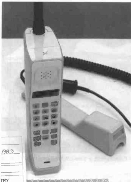
An early "cell phone" by Motorola, the "TacTek." Selling for \$3,995 in 1983, it weighed 16 oz. It was based on the original Motorola "DynaTac," developed in 1973, which weighed 3 lbs. It contained 30 circuit boards, and you could talk for up to 35 minutes on a charge. DynaTac stood for "Dynamic adaptive Total area coverage."
