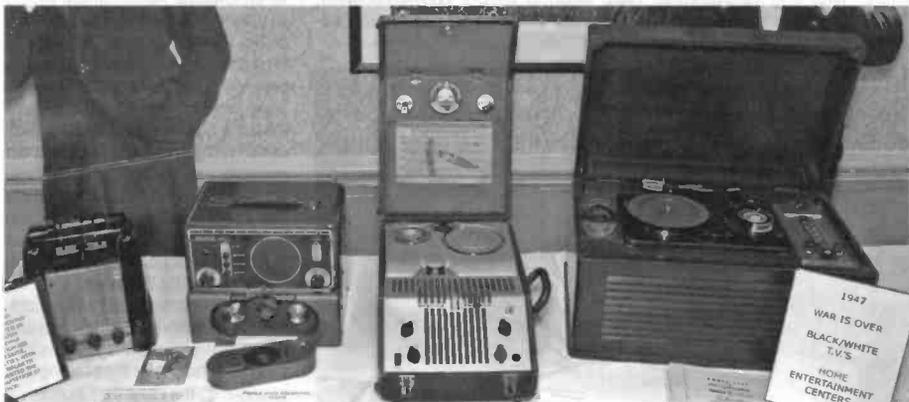
*Jack LaVelle offered this selection of wire recorders in the contest. Left is a 1930s/40s RCA wire recorder that used a cartridge containing the wire reels. Second from the left is a Pierce 260 wire recorder made by F.D. Thomas company in the 1940s. Next is the relatively common, Webster Chicago wire recorder, also from the 1940s. On the right is the "Superheterodyne Radio Receiver with Wire Recorder" by Silvertone.*
