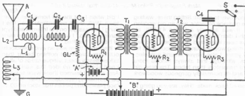
Figure 6. Three-tube Cockaday circuit diagram from Sidney Gernsback's "Radio Encyclopedia." Missing from Art Redman's set is the feedback provided by L4's connection to the plate of the left-most vacuum tube.
