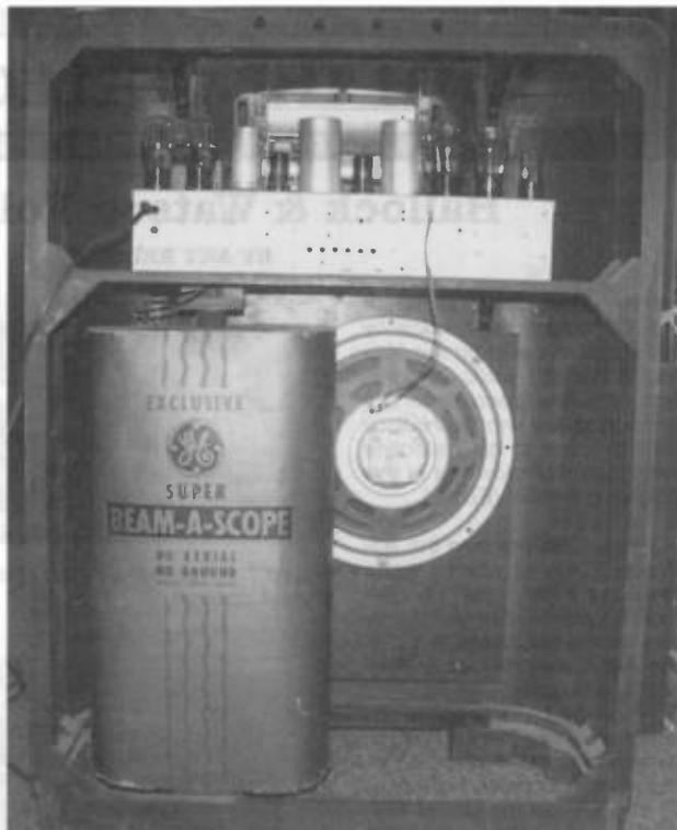
Figure 2. Rear view of the 1939 GE H-87 console. The large chassis and "Beam-A-Scope" are prominent.
