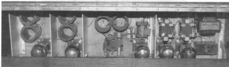
Figure 5. A view inside the cabinet of the Cockaday LC-27 components.
