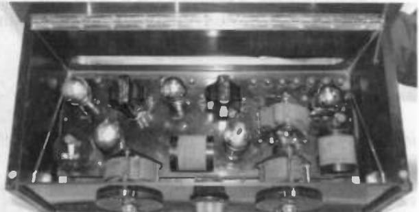
Figure 3. An inside view of the cabinet of the Hallock & Watson Model AW-5 showing the neat component layout.
