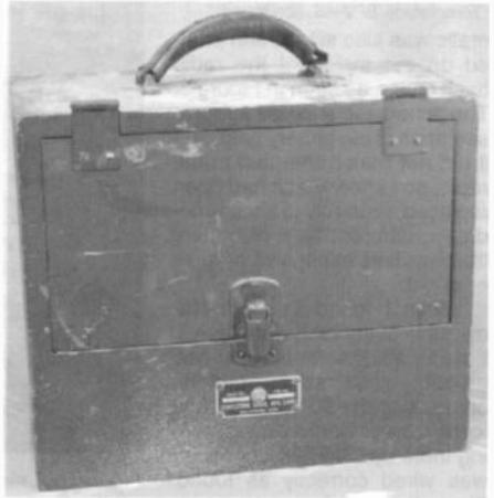
Figure 4. The case is a simple plywood box painted a military olive drab.
