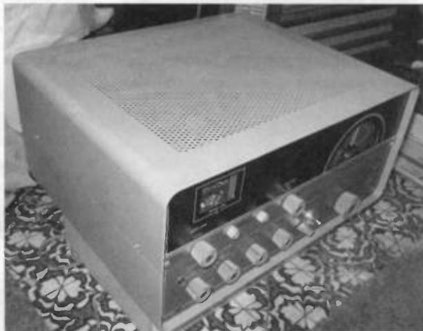
Figure 2. The repaired Hallicrafters HT-37 transmitter, also purchased at the auction.
