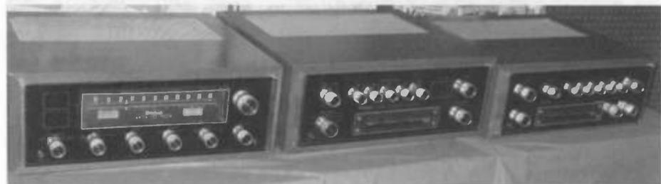
Three McIntosh items — left to right, an FM tuner, an MA 6200 integrated amp, and a C-33 pre-amp, all in wood cases.
