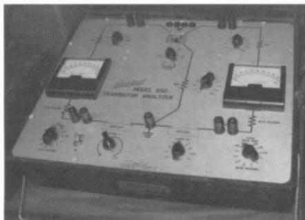
An early Hickok 850 transistor analyzer.
