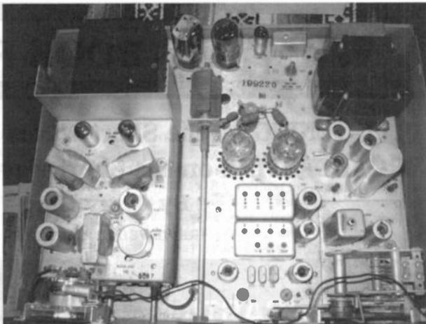
Figure 3. Hams will skip a heart beat when they see a chassis this clean. The two 6146 output tubes can be seen in the upper center of the photo.
