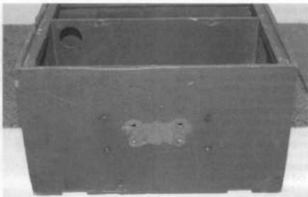
Figure 12. The cabinet showing extra holes drilled for mounting the replacement handle and door switch.
