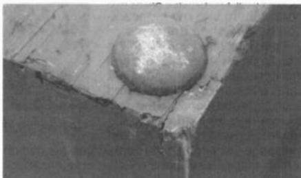
Figure 11. A rusted steel foot on the bottom of the cabinet ready to be removed and bead-blasted.
