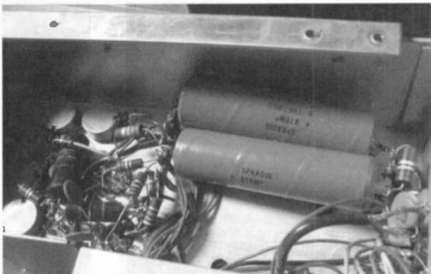
Figure 4. New electrolytic capacitors, upper right, shown installed in the transmitter chassis.
