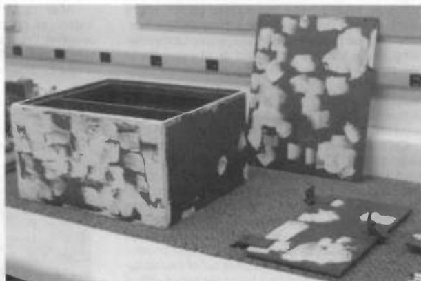
Figure 14. The holes and dings are ready for sanding and paint.
