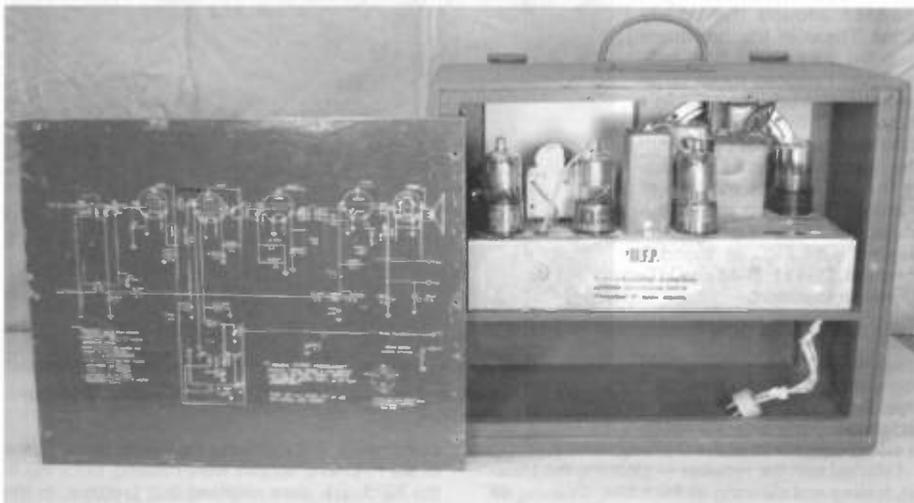
Figure 17. An interior view of the finished product with the back cover off showing the schematic on the inside.
