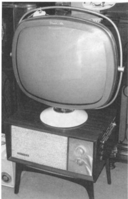
*This Philco Predicta, selling for \$225, is the model with the remote console (bottom) which can be separated from the picture tube. A long, flat, multiconductor cable connects the two units.*
