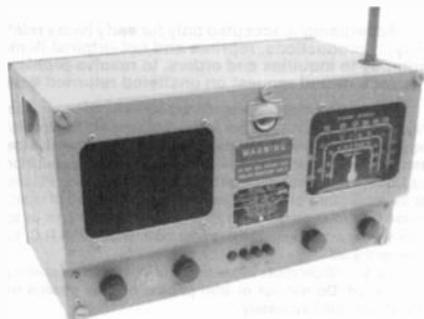
Inside the chassis are spare socketed tubes for each active tube in the set. Unfortunately, the prior owner made off with the spare 6E5 eye tube. It plays very well!
