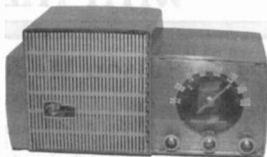
**GENERAL ELECTRIC MODEL 431** – This 6-tube table radio was manufactured in 1955 by GE and sold for \$45. A similar radio was issued as Model 621. Both radios were broadcast sets with Civil Defense markings. (Clark Trissell – Lincoln, NE)
