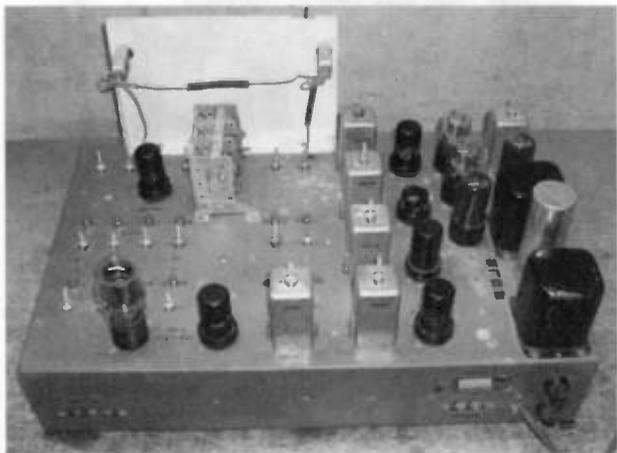
Figure 2. An interior view of the Model R-138 chassis where both tubes and adjustments had corresponding ID labels painted on.
