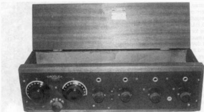
**CROSLY MODEL XJ** – Sold by the Crosley Radio Co. of Cincinnati, Ohio, in 1923, this 4-tube battery receiver uses all Type 01-A tubes. It tunes using two "Book Type" tuning condensers made famous by Crosley. (Clark Trissell – Lincoln, NE)
