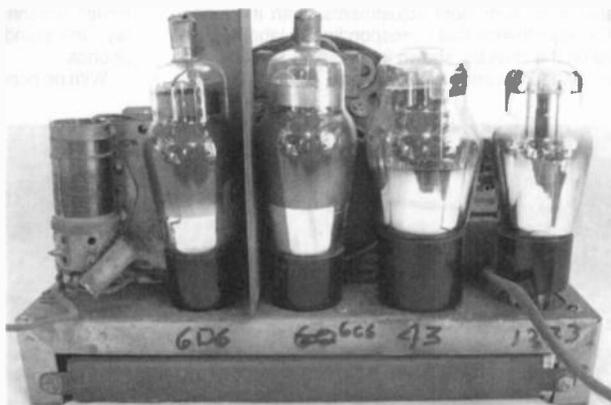
Figure 6. A rear view of the chassis showing the horizontally mounted 220-ohm, filament, voltage dropping resistor on the bottom.
