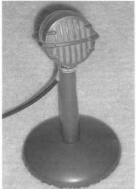
Figure 3. The Astatic Model W80 microphone (original) shipped with the Silvertone 7086.
