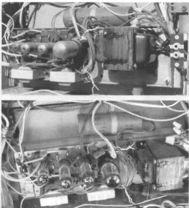
Figure 8. The amplifier chassis shown before restoration, above, and after restoration, below. Note the general clean up of the chassis and components, and the rebuilt cardboard electrolytic capacitor, seen above the vacuum tubes and transformer.
