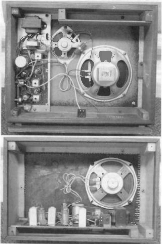
Figure 7. Interior views of the remote speaker cabinets, the large, above, and the small, below, showing the speakers and FM receivers.
