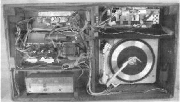
Figure 9. A rear view of the restored unit with the rear cover removed. The added MDS unit is on the lower left.
