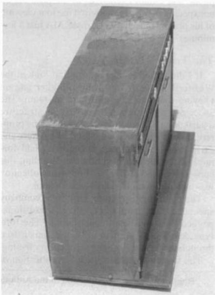
Figure 2. End view showing water damage.
