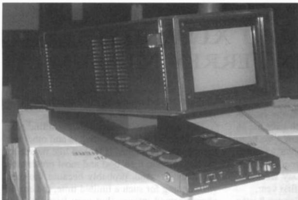
*This is a very collectible Sony Trinitron portable color television set. Marketed in 1980, Sony claimed that it was "the smallest Trinitron color TV in the world, with a 3.7-inch diagonal picture."*
