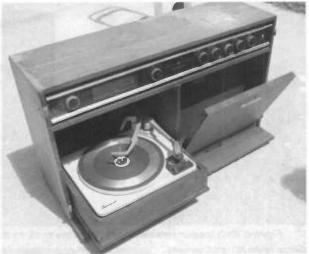
Figure 3. This open view of the cabinet shows the water damage to the top veneer. The compartment to the right is for record storage.
