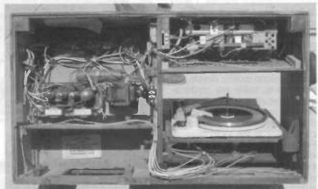
Figure 5. A pre-restoration rear view of the system with the rear cover removed. The location for the missing MDS unit is on the lower left.
