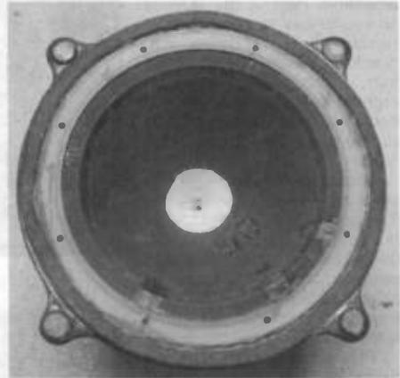
Figure 8. The armature shaft is attached to the center of the cone.
