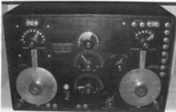
Figure 8. The SE-712A receiver.
