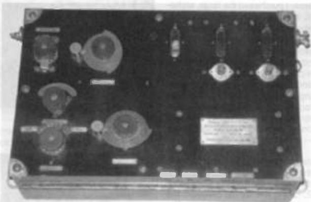
Figure 9. The Western Electric SCR-75 radio aircraft receiver.
