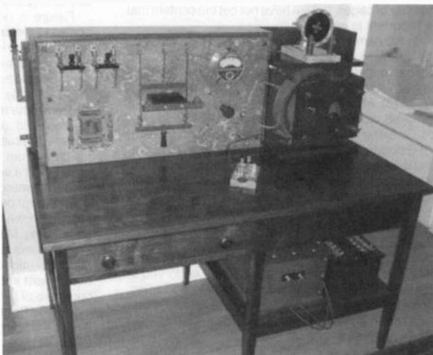
Figure 1. Clapp-Eastham 1-Kilowatt Spark Transmitter.
