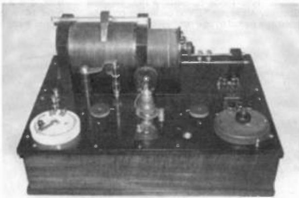
*Figure 7. Fleming Valve & Radioson electrolytic detector receiver.*
