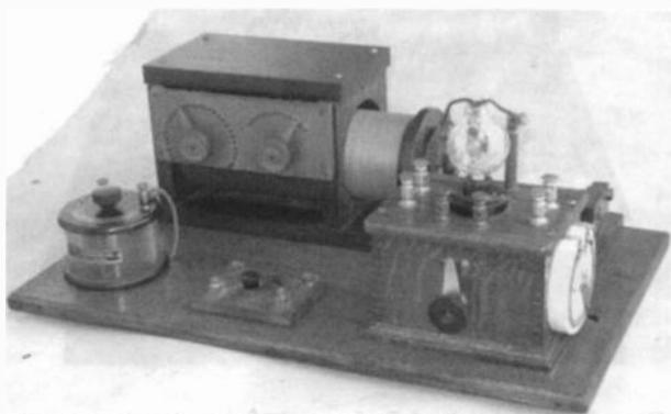
Figure 5. A Spherical Audion breadboard radio.
