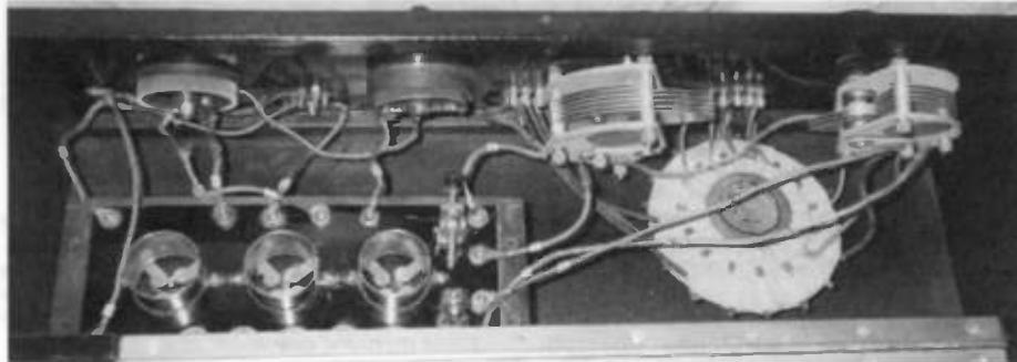
Figure 3. The components inside the set can be seen here. The 3-tube unit on the left actually is a sealed module and weighs about seven pounds! The crystal detector also is mounted on this unit.
