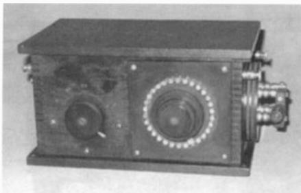
Figure 2. Clapp-Eastham Blitzen receiver.
