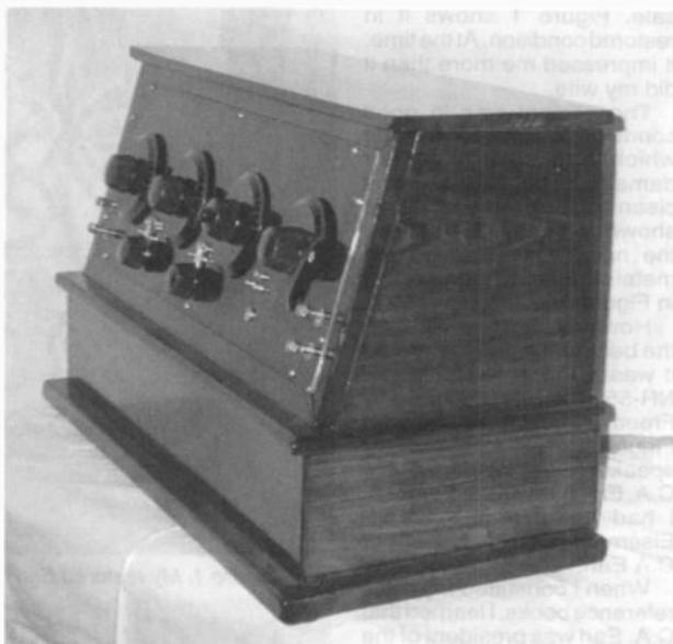
Figure 5. My restored Ozarka set. Unfortunately, I am still missing the right dial and selector switch.
