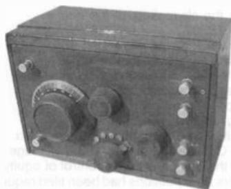
**CROSLLEY MODEL 50** – This 1-tube regenerative receiver was manufactured in 1924 by the Crosley Company of Cincinnati, Ohio. Its regeneration was achieved by adjusting two spider-web coils with the knob just above the tap-switch on the panel. (*Dave Crocker – Mashpee, MA*)
