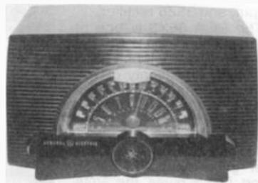
**GENERAL ELECTRIC MODEL 409** – This AC-DC table radio in a plastic case was manufactured in 1952 by GE. It operates on the following seven tubes: (3) Type 12BA6, (1) Type 12AT7, (1) Type 12AV6, (1) Type 35Z5, and (1) Type 19T8. It tunes with two thumbwheel knobs on either side of the front plastic extension. (*Clark Trissell – Lincoln, NE*)
