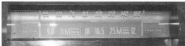
*The dial scale is marked for the 9 to 12 kHz (31 to 25 meter) shortwave band.*
