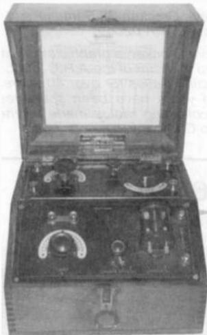
**B.T.H. Radiol 1** – This one-tube crystal set was manufactured in 1923 by the British Thompson-Houston Co., Ltd., of Coventry, England. It is stamped "Wireless H.F.-Valve Receiver." It uses a double crystal detector under a transparent holder with two adjustable knobs. The tube is mounted inside under the panel. (*Jim Taylor – Winton, Bourmemouth, England*)
