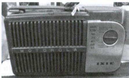
*Not all battery sets were from the 1920s. This mid-1950s, portable Motorola Pixie sold for \$45. It was unusual in that three of the four tubes were subminiature tubes, about the size of a pencil.*
