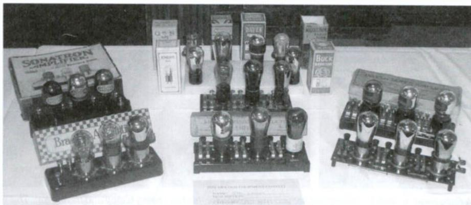
Joe Knight entered this display of 3-tube, resistance coupled, audio amplifiers from 1925 and 1926 in the old equipment contest. The manufacturers, left to right, are Sonatron, Bradley-Amplifier, DeJur, Kelford, Daven, and Muter.
