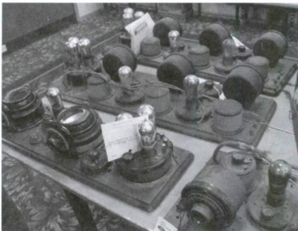
Several Atwater Kent breadboards were included in the sale. The Model 9, the No. 4445, front left, is the early version. It can be identified by the green painted tube unit, battery terminals, and the Type 11 and Coupled Circuit tuners. It sold for \$1,700. The later versions of the Model 9 had a battery cord and brown painted tube units. The Model 9C had tuning capacitors instead of the Type 11 and Coupled Circuit tuners.
