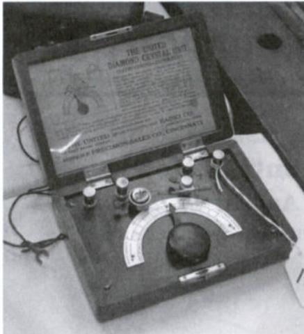
This small crystal set called the "United Diamond Crystal Unit," manufactured by the United Metal Stamping and Radio Co., Cincinnati, Ohio, sold for \$225.
