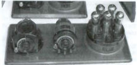
*The breadboard Model 8, No. 4325, uses the same 5-tube unit as the Model 5.*
