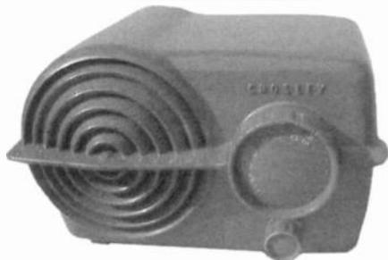
**CROSLY MODEL 11-115U** - This maroon, plastic, table radio was manufactured in 1951 by the Crosley Radio Manufacturing Company of Cincinnati, Ohio. Its 5-tube chassis tuned the broadcast band only. The whole 11-series of "Serenader" table radios came in assorted colors. (Dave Crocker - Mashpee, MA)
