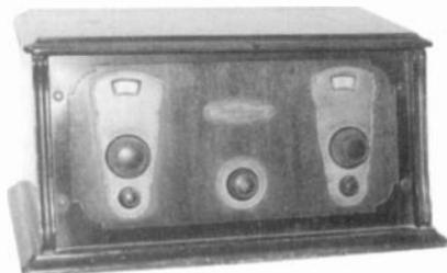
**FREED-EISEMANN MODEL 30** - The Freed-Eisemann Corporation of New York manufactured this 6-tube battery set in 1926. It operates with the Neutrodyne circuit using two tuning dials. (Clark Trissell - Lincoln, NB)
