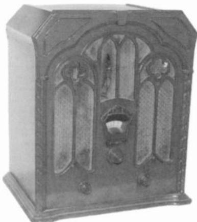
**MAJESTIC MODEL 311** - Built in 1932 by the Grigsby-Grunow Co., this tombstone table radio uses the following seven tubes: (1) Type 80 rectifier, (1) Type 47, (1) Type 55, (1) Type 56, and (3) Type 58. (Clark Trissell - Lincoln, NE)
