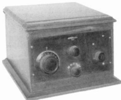
**CROSLY MODEL 51-S** - This 2-tube regenerative receiver with binding posts inside is the standard Model 51 in a deluxe cabinet. It was manufactured by the Crosley Radio Corporation of Cincinnati in 1925. (Clark Trissell - Lincoln, NE)
