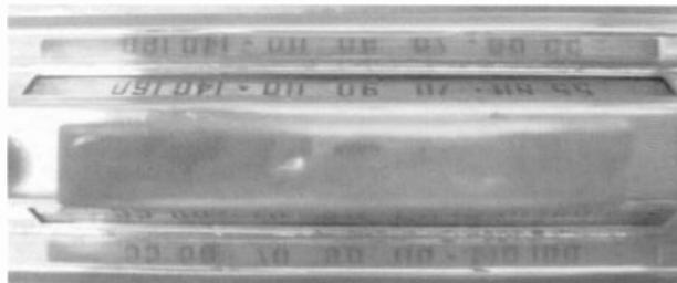
Figure 3. A close look at this photograph taken from above the handle shows a dial with markings from 55 to 160 both above and below the handle; thus, a dial can be seen from both the front and rear of the set.
