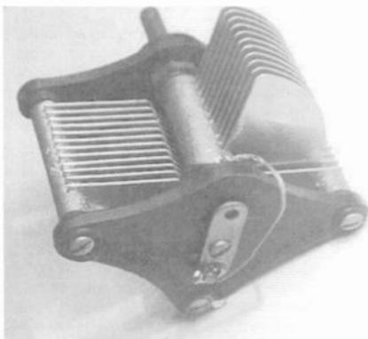
Figure 6 Added connection to the ZR-4 Tuning Capacitor.
