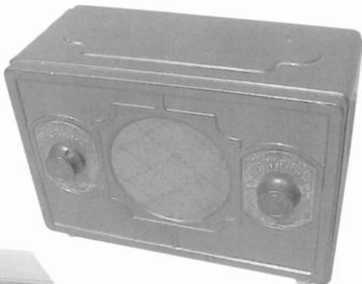
**PHILCO MODEL 50-524** – This 5-tube receiver of 1950 was manufactured by the Philco Corp. of Philadelphia. It is one of the many “Transitone” radios which Philco offered in the 1950s. It uses one each of the following tubes types: 7A8, 12BA6, 14B6, 50L6, and 35Z5. It tuned the broadcast band only. (*Clark Thissell – Lincoln, NE*)
