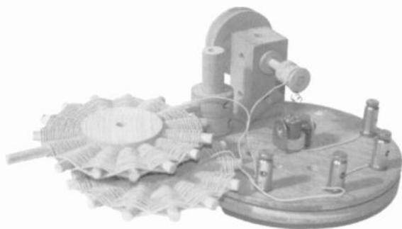
**RADIODYNE MODEL WC10** – This 5-tube receiver was manufactured by the Western Coil and Electrical Co. of Racine, Wisconsin. In 1923, it sold for \$150, less tubes, batteries, and speaker. (*Wally Worth – Wollaston, MA*)
