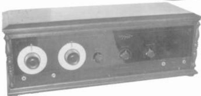
**HYPOWR SUPERHET** – This 8-tube battery superhet from the mid-1920s is identified as HyPower Super on the panel, but inside, it uses all Victoreen coils and IF transformers. The tubes are Type 201A. (Ray Chase – Plainfield, NJ)
