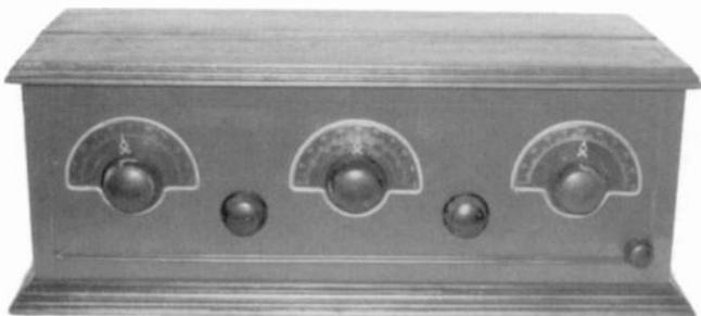
**STEWART-WARNER MODEL 300** – This battery-operated, 5-tube receiver was manufactured in 1925 by the Stewart-Warner Speedometer Corp. of Chicago. The tubes used in the circuit are the following types: (1) 200, (3) 201, and (1) 112. The wood cabinet has a metal panel. (Clark Thissell – Lincoln, NE)
