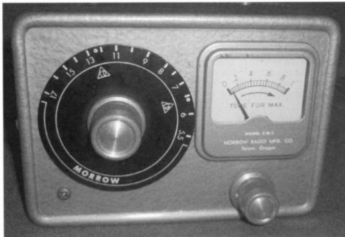
drum dial mechanism, unlike the more common model MBR-5. The compact MB-6 measures 4 x 4 x 7 inches (HWD) with three of the 13 tubes mounted sideways. The set is known for its extraordinary stability, outperforming all its lower priced competitors like the Elmac models PMR-7 and PMR-8.
