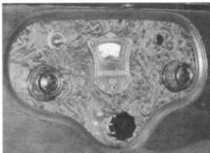
*The wooden front section of the Kiel table pulled down reveals the wood-grained control panel of the Atwater Kent Model 60. Note that the bottom tuning knob is incorrect.*
