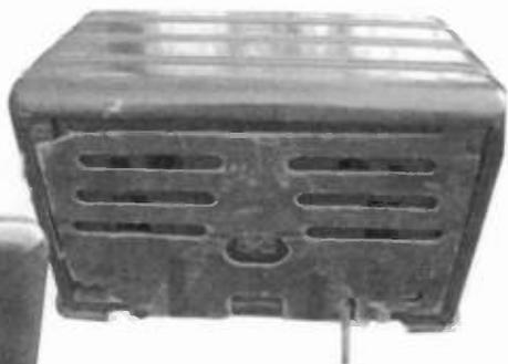
**RCA 56X3** - Circa 1946, tube line up: 12SG7, 12SK7, 12SQ7, 35L6GT and 35Z5GT. Five-inch speaker has a nice tone. It is a very sensitive set, even though a simple one with just the broadcast band. Has high/low tone control. (*Paul Buresh, Needham, MA*)
