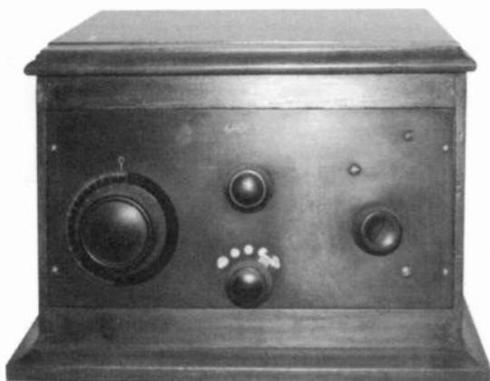
**CROSLY MODEL 51-S** - This two tube battery receiver was manufactured in 1925 by the Crosley Radio Corporation in Cincinnati, OH. The "S" in the model number means "Special." The chassis and panel are the same as the standard Crosley Model 51, except for having a variable plate tuning condenser instead of the older "book" type tuner and a larger more deluxe cabinet. (Dave Crocker, Mashpee, MA)
