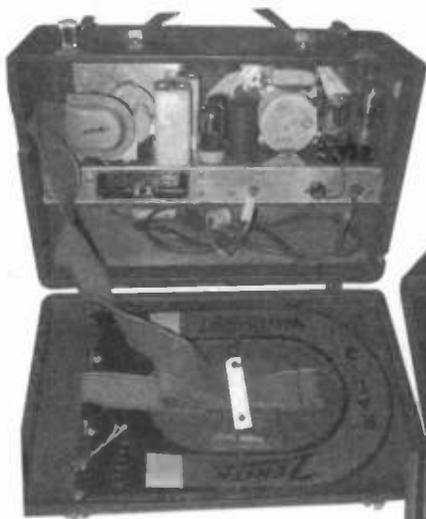
**Zenith model 6G501L** - One of the many Zenith portable radios made in the 1941. The chassis number is 6A19 with six tubes and it operates on both AC and DC power. It is leatherette covered and the front uses a rare wood bezel. The wave magnet was also included. (Phillip Sandweiss - Tombstone, AZ)
