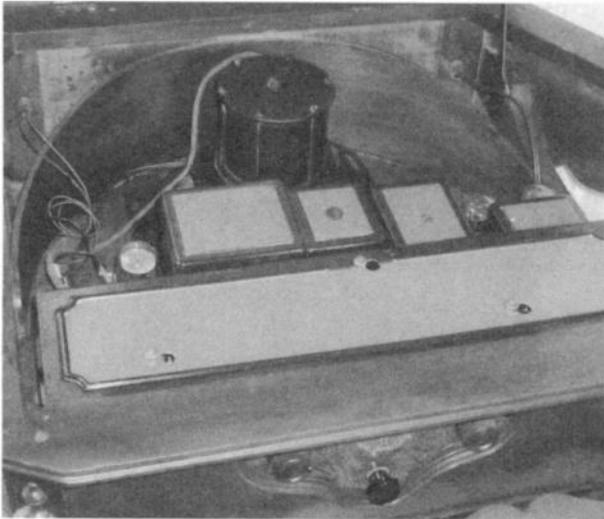
*With the Kiel table lid lifted, you can have access to the Atwater Kent 60 chassis and speaker.*
