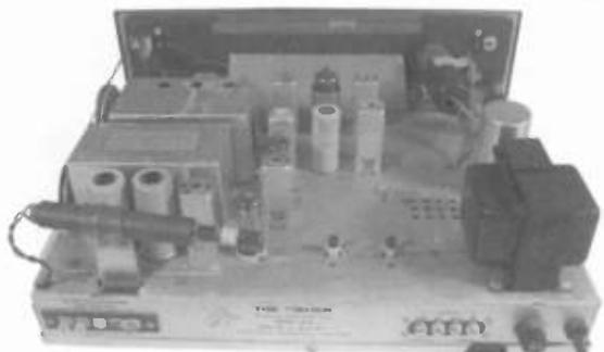
**Fisher model 100-R AM/FM Tuner** - This was manufactured in the 1960 to 1961 era. Has both AM and FM bands but is not stereo. It had separate outputs for both the AM and FM. Not often seen. (*Woody Korman-Los Angeles, CA*)
