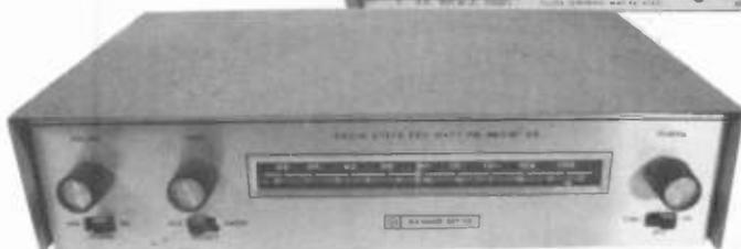
**Westinghouse model RA DA battery set combination** – The RA was the receiver tuner and the DA was the detector amplifier. Sometimes seen as the combined RC unit. *George Geiger – Sioux Falls, SD*
