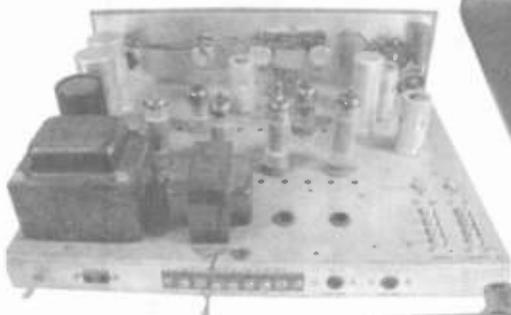
Lafayette model 236A stereo amplifier - Uses 4 EL84 output tubes. Note one of the output transformers is missing. *Robert Middleton, Nashville, TN*
