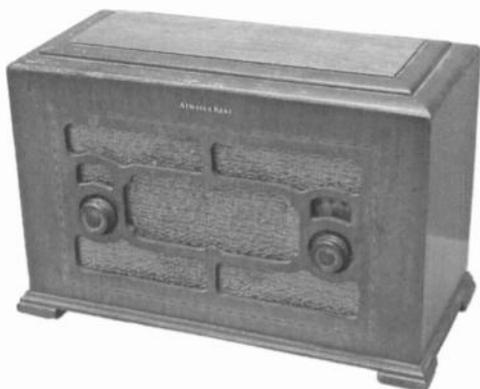
**Atwater Kent model 155** – This wooden table radio was manufactured in 1933. It has five tubes and receives the broadcast band only. Dave Crocker, Mashpee, MA
