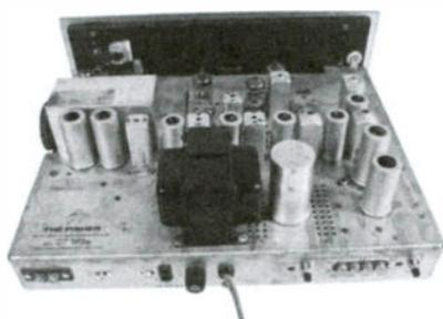
**Fisher FM-100-B FM Tuner** – This 12-tube FM tuner from 1963 featured variable muting, signal meter, and stereo indicator light. Alvin Savella, Little Neck, NY
