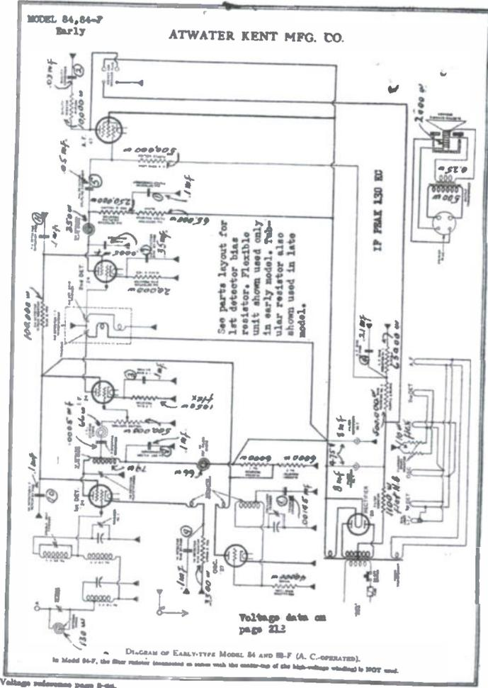
Figure 1. Schematic of the "early" model 84 receiver
