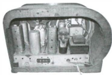
**Philco Model 38-10 Radio** – This radio was made in 1938 and contains five tubes. A multiband set, it covers AM and shortwave bands. AC powered. Marty Olson, Kansas City, KS
