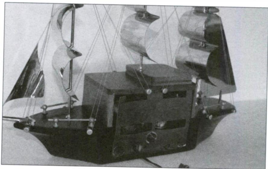
*Rear view of my Majestic Melody Cruiser. It had the original back with its anti-shock seals still located over the back hardware, which screw into the electrically hot chassis.*
