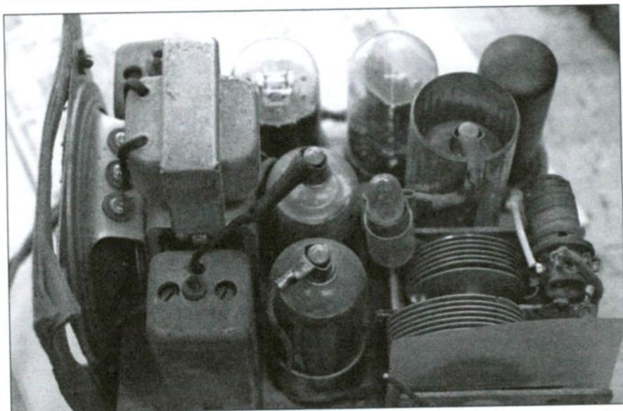
*The speaker of my Charley McCarthy is original and in perfect condition. Note that in chassis II the 455 kHz IF transformers are in shield cans, unlike the chassis I version. Note the L49-B ballast resistor in a sealed metal tube.*
