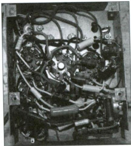
*The Charley McCarthy chassis after replacing all capacitors. Note that I used metallized polyester film capacitors, and the Orange Drop is a 0.01  $\mu$ F 1600V capacitor across the AC power line.*
