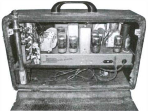
**Zenith model 8G005TZ1** – A Zenith Transoceanic model made in 1948. Powered by AC, DC, or battery. Covered AM and shortwave bands. Denny Bayer, Lincoln, NE
