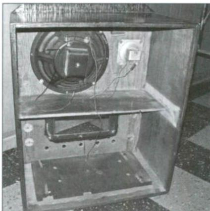
*The rear of the custom-built tombstone cabinet showing the 10-inch speaker and the piece of Plexiglas I glued in place from the inside to protect the original Fisher dial scale glass on the chassis.*
