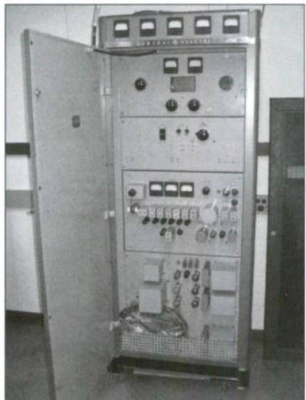
*A General Electric type BT-1-B FM transmitter, circa 1940s. Output 250 watts, 88 MHz–108 MHz. It's still in operation.*
