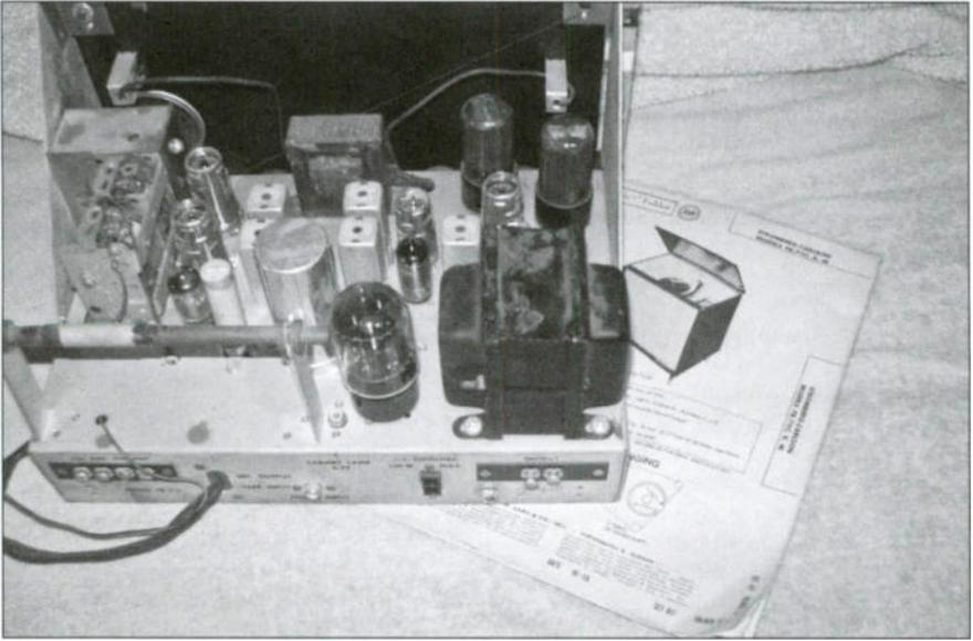
*Note the decent sized output transformer on the chassis in the center towards the front. This transformer is driven in "push-pull" by the two 6V6GT output tubes, also visible. An illustration of the original console lies partially beneath the chassis. One could easily build a very nice set, about 1 cubic foot in size, around it.*
