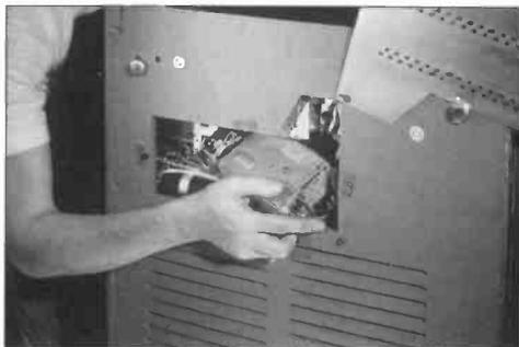
**Inserting UHF Tuner** – A service tech installing the optional UHF frequency tuner.
