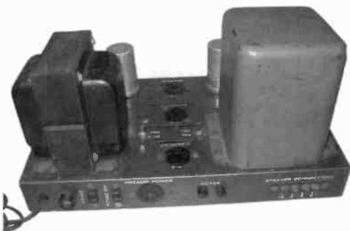
**Eico HF-50 Audio Amplifier** – The power output from this mono block audio amplifier was 60 watts. Output tubes are 2 x EL34. Made in 1959. The HF-50 used a Chicago output transformer and the HF-60 used a Accrosound output transformer with an output of 60 watts. Karl Breen, Fargo, ND
