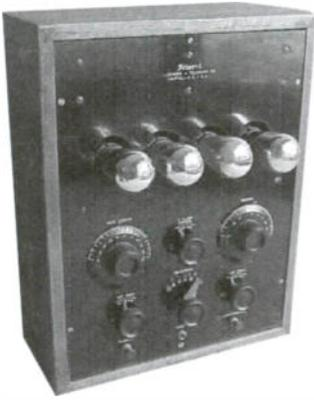
**Federal Model 135** – This four tube receiver was made to fit into the cabinet of your replaced photograph. It was manufactured in 1924 by the Federal Telephone and Telegraph Co. of Buffalo, NY. Dave Crocker, Mashpee, MA.
