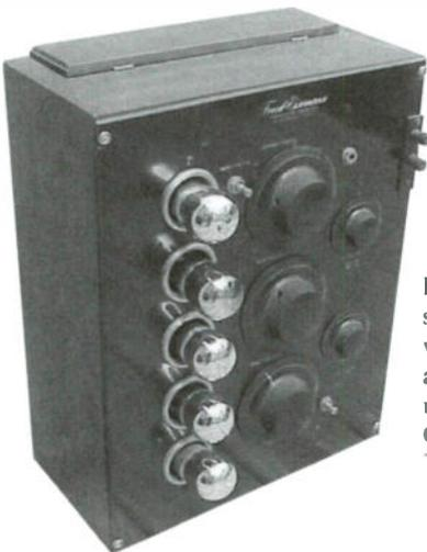
**Freed-Eisemann Model NR-205** – This seldom 5 tube receiver of 1924 was produced to replace your phonograph and fit into its cabinet. The controls were under the flip-top cover at the top. Dave Crocker, Mashpee, MA.
