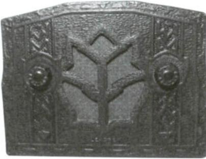
**The LeWol "Lavore"** – This 4-tube TRF set was manufactured by one of the lesser-known radio companies; The LeWol Manufacturing Corp. 844 W. Adams St., Chicago, IL. Its tube line up is conventional and typical for the early 1930s. The tube complement consists of one each of the follow types: 6D6, 6C6, 43, and 25Z5. The cabinet is covered with leatherette and features ArtDeco designs. Ray Bintliff, Acton, MA.
