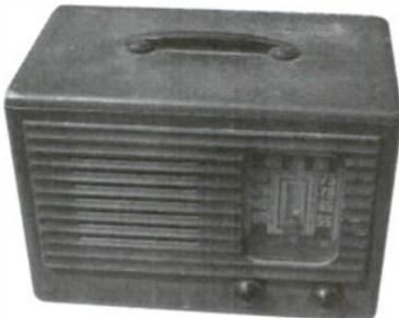
**Emerson Model 334** – This 1940 table radio operated with a 5 tube chassis. The cabinet was know as an “Ingraham” cabinet type. It sold in 1940 for \$65.00. Dave Crocker, Mashpee, MA.
