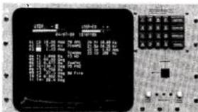
The **RCS-1 Remote Control System** combines microprocessor technology with simplified operation. Features include direct interface boards for antenna monitors, patented remote modulation bargraph, automatic logging, and synthesized speech telephone interface. The modular design allows the customer to plug in additional input or control boards to expand remote control capabilities even after the system is operating in the field.
