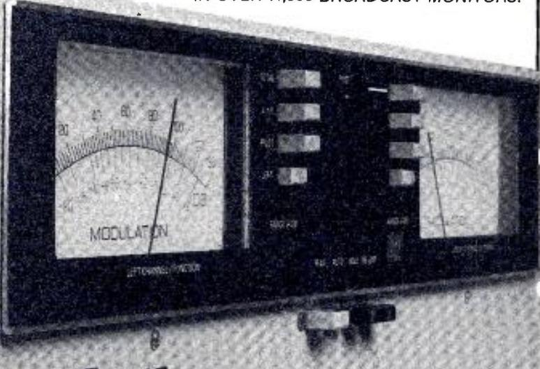
The FMM-2/FMS-2 series monitors provide an even greater degree of precision measurement and stability than ever before... Specifications, which include better than 90 dB S/N, less than .01% maximum THD and IM distortion, and 70 dB stereo separation, make Belar FM monitors the most accurate available today.
