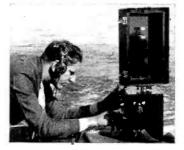
IN SEARCH of a new transmitter site, KGER, Long Beach, Cal. is taking field measurements on land and water throughout Southern California. Here is Chief Engineer Jay Tapp aboard a yacht off Long Beach, taking measurements.
