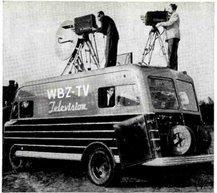
THIS NEW MOBILE television control room is scheduled for early fall delivery to Boston's first television station, WBZ-TV. It houses all necessary equipment for a two-camera television pickup operation. Two image orthicon cameras and the microwave relay unit are mounted on top of the vehicle.
