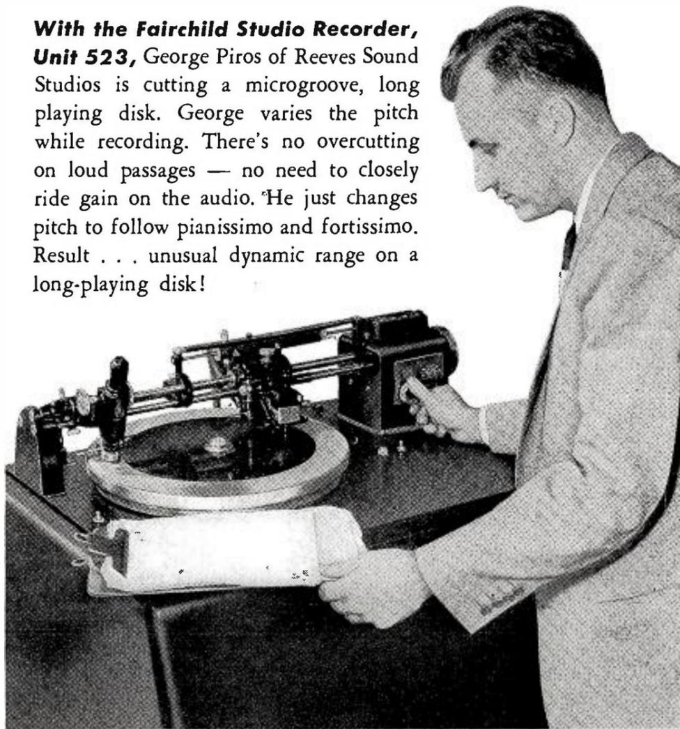
The Fairchild Studio Recorder Unit 523 offers continuously variable control of cutting pitch operable while recording. You don't have to change feed screws, belts, pulleys or other mechanisms. Simply rotate a conveniently located knob for smooth and vernier control of cutting pitch. This gives you continuous and instantaneous variation of pitch from 80 to over 500 lines per inch during the actual recording.
