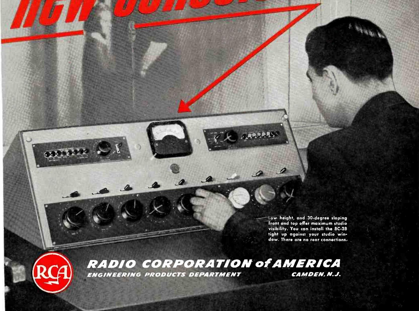
Low height, and 30-degree sloping front and top offer maximum studio visibility. You can install the BC-2B tight up against your studio window. There are no rear connections.
