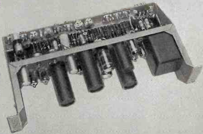
NEW VIDEO DISTRIBUTION AMPLIFIER TA-3A. Feeds up to 3 low-impedance lines from single high- or low-impedance source. Has extended low- and high-frequency response. 40-db isolation between output lines. Excellent linearity and gain characteristics. TA-3A is good for color.
