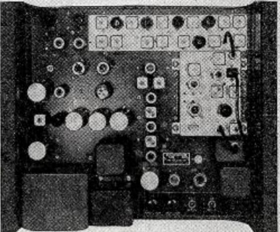
The Type TRC-1 Color Rebroadcast Receiver has been designed specifically to meet the requirements for a high-quality receiver for use in direct pickup and rebroadcast of black and white and color signals.
