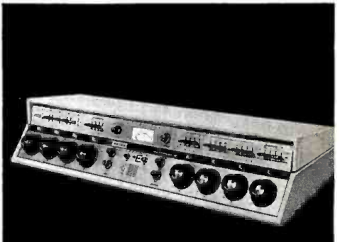
Gateway II Console – 8 monaural mixing channels from 18 inputs. Provides for remote announcer operation of studio mike channel.
