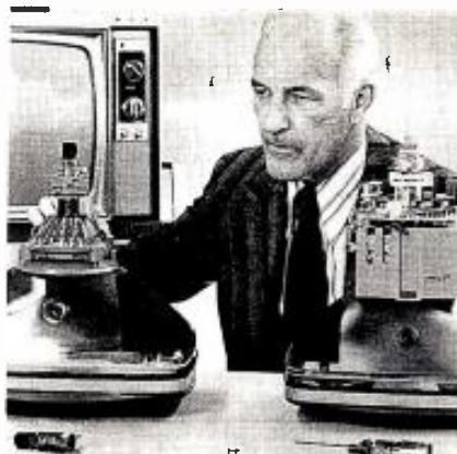
Colorful color. RCA engineer Hollis Carter with the firm's new in-line color-tube system on the left with the current and more complex color-tube system on the right.
