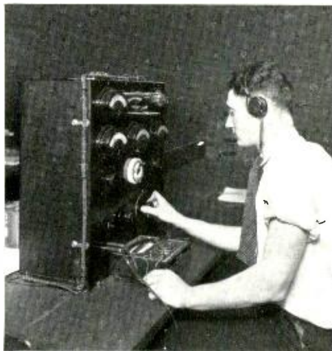
At the repeater test-boards Eugene C. Russell makes electrical tests on the 101-D tube
