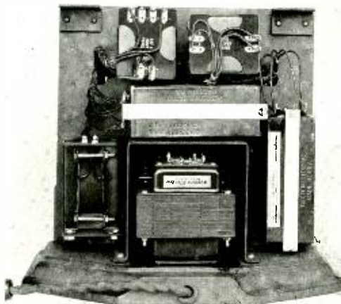
Inside view of amplifier, showing power transformer
