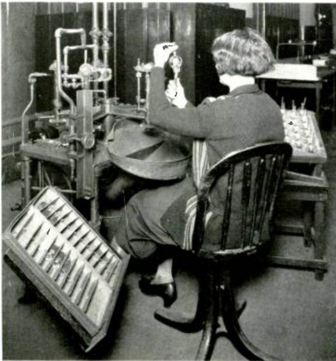
Mrs. Martha Frykholm operates the glass-sealing machine which seals the mount into its bulb
