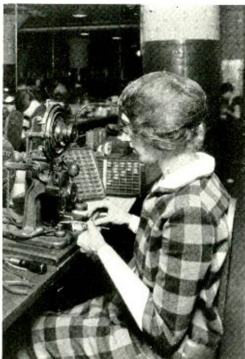
Miss Juliette Charpin manipulates the electric welding of the grid
