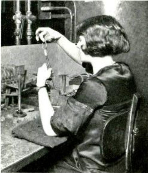
Miss Lena Sproat "raising the arbor" on the stem press of the 101-D tube
