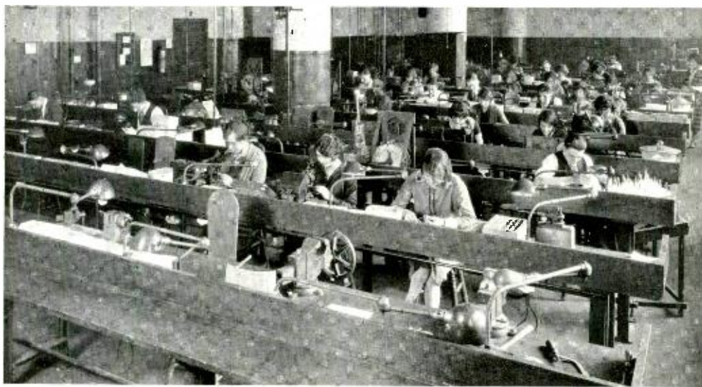
A section of the Assembly Department, where the elements of the tube are constructed and attached to the glass stem unit
