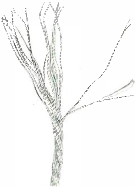
Fig. 1—Old cord conductor, showing construction of tinsel threads and method of stranding
