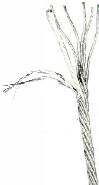
Fig. 2—New conductor, showing double ribbon tinsel threads twisted around a central core of bare cotton thread
