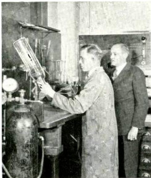
E. D. Deery and H. W. Weinhart completing the glass work on a photoelectric cell for special research
