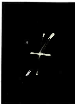
Fig. 3—Oscillograms for the 9-A amplifier—a single-stage push-pull circuit using two 205-D tubes with a 350-volt plate battery
