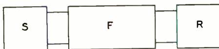
Diagrammatic representation of an electrical filter F, receiving current from source S, and delivering to receiving element R
