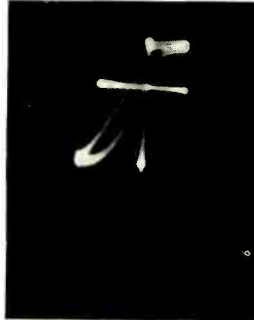
Fig. 2—Oscillograms of output vs. input for the 8-B amplifier. In the last one of its three stages was a 205-D tube with a 350-volt plate battery
