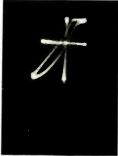
Fig. 2—Oscillograms of output vs. input for the 8-B amplifier. In the last one of its three stages was a 205-D tube with a 350-volt plate battery
