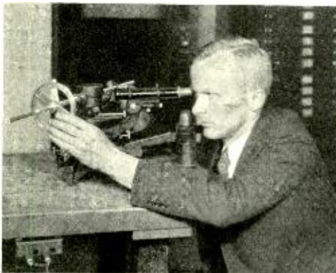
Figure 8—D. D. Foster using the optical goniometer to fix the orientation of a single-crystal wire
