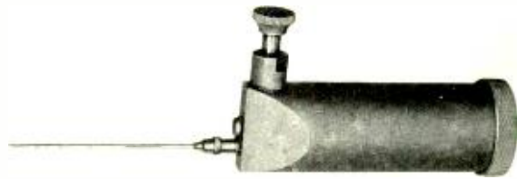
Grease gun for cam-shaft bearings of the sequence switches
