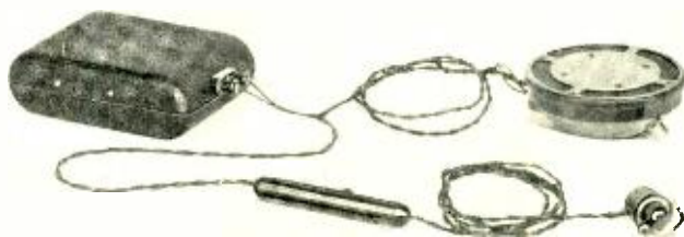
The 6033-B Audiophone is similar to the 6034-A, but the transmitter is hung on the coat-lapel and batteries are carried in the pocket
