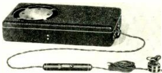
The 6034-A Audiphone requires no vacuum tubes. In the case are the transmitter and batteries
