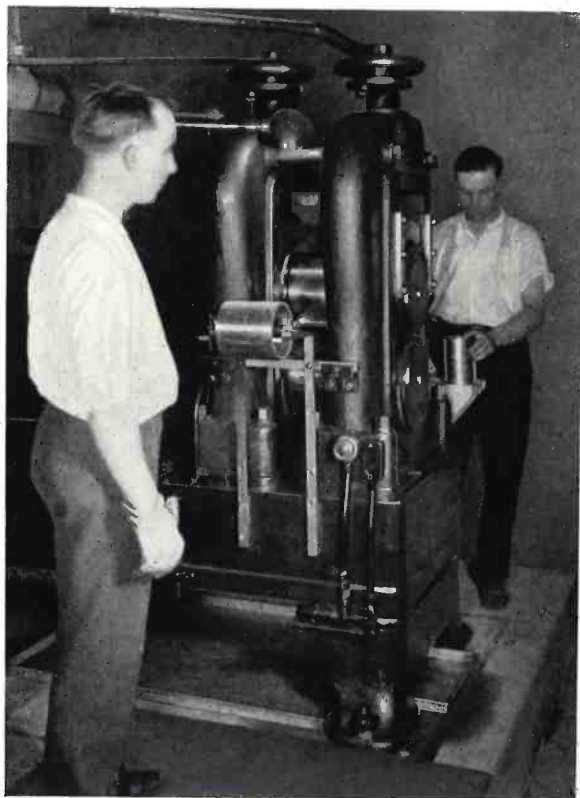
R. J. Riley and J. M. Artiges roll out a sheet of diaphragm stock
