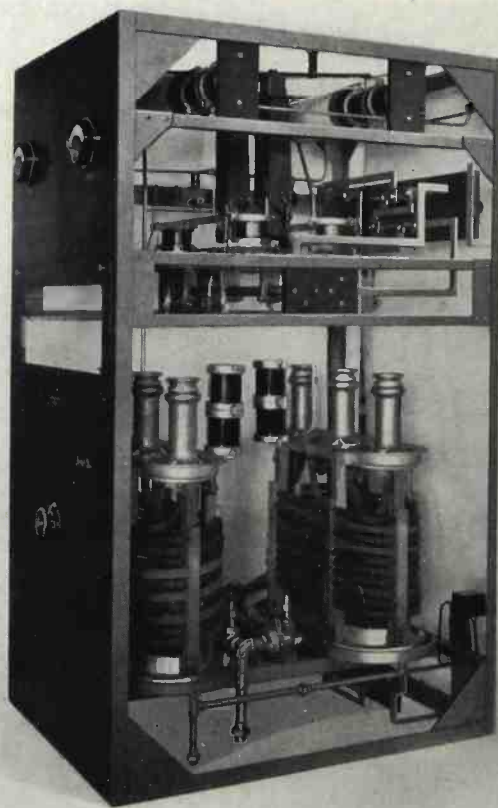
A side view of the last-stage tube unit before the tubes were placed in their jackets
