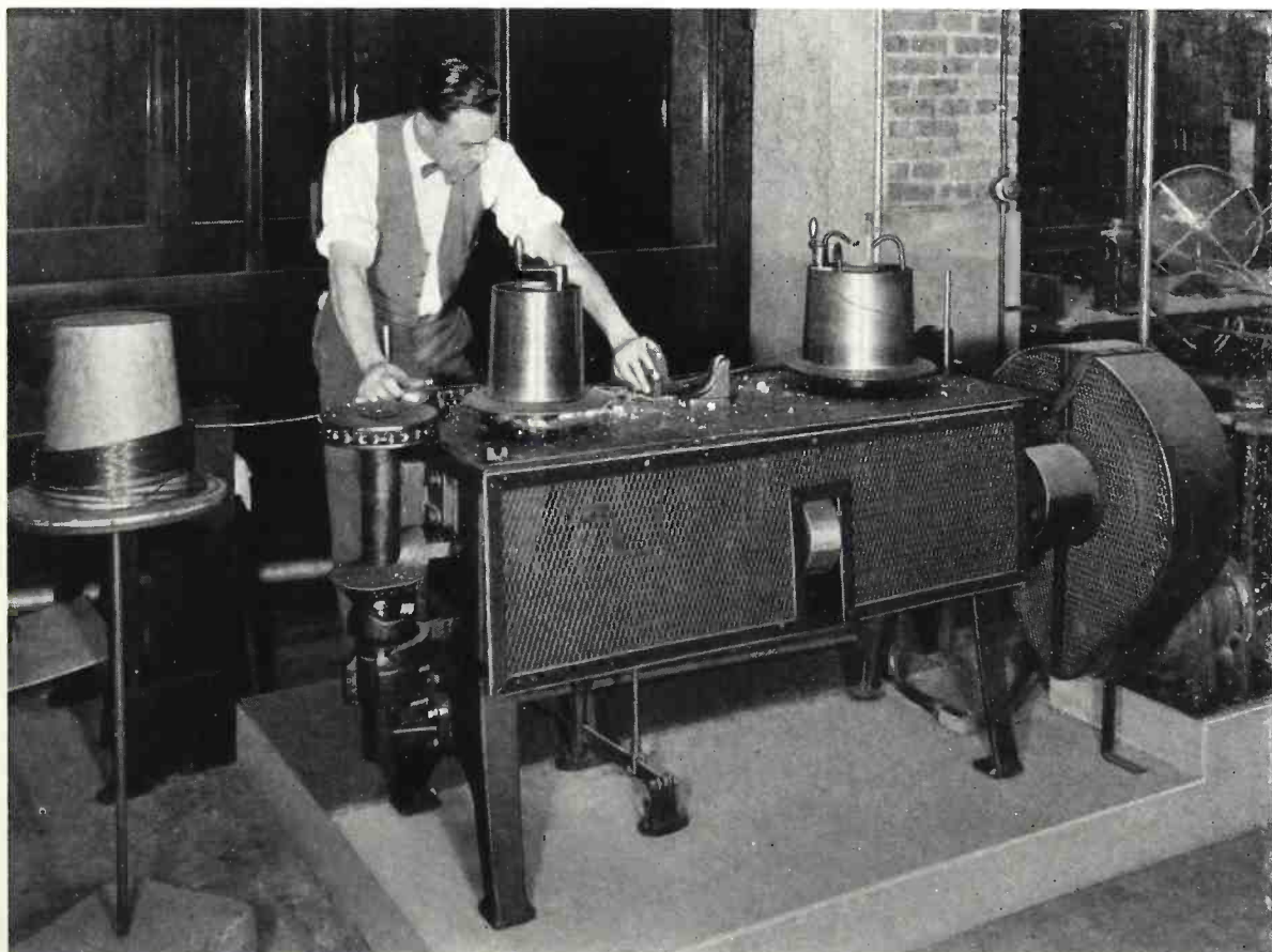
The wire-drawing bench is one of the oldest of metal-working machines. Its modern counterpart in our Laboratories is operated by D. Wallace
