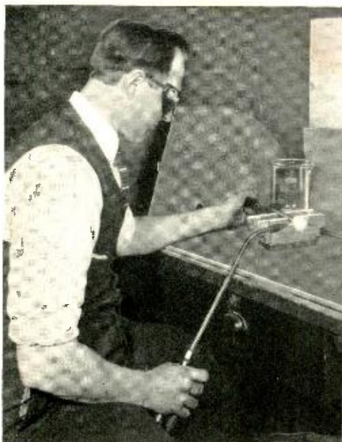
Fusing a platinum rod with oxyhydrogen torch to remove bubbles and air pockets
