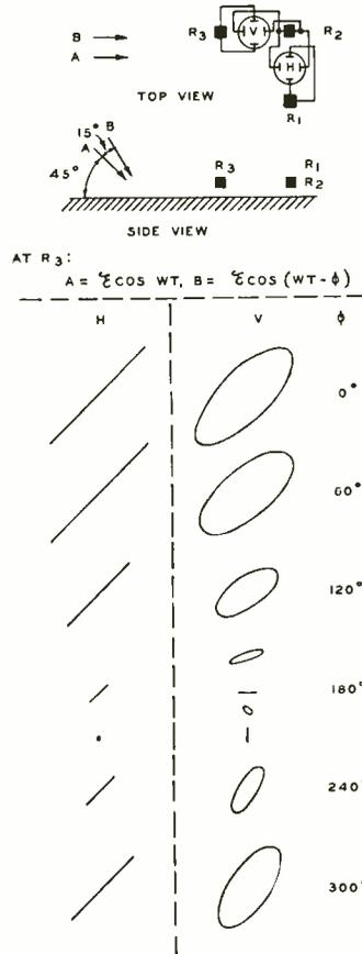
Fig. 4—Illustration of fading effects due to reception of two waves at slightly different angles
