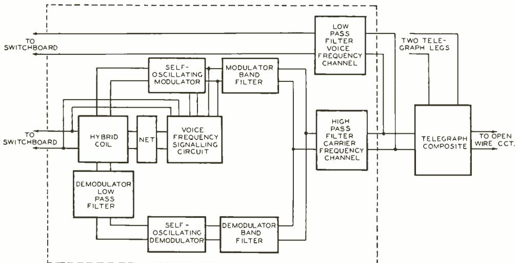
Fig. 1—Equipment symbolized inside the dotted lines is that for the D-1 System
