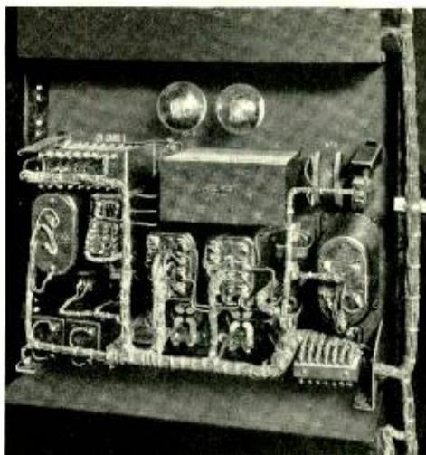
*Reverse of lower panel, showing the modulator circuit*
