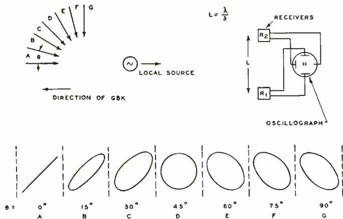
Fig. 1—Arrangement of receivers and local oscillators for determining horizontal-plane angle of reception
