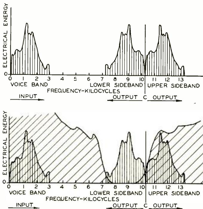
Fig. 4—Above, the location on the frequency spectrum of input and output currents of the modulator; below, how the band-pass filter eliminates all but the lower side band
