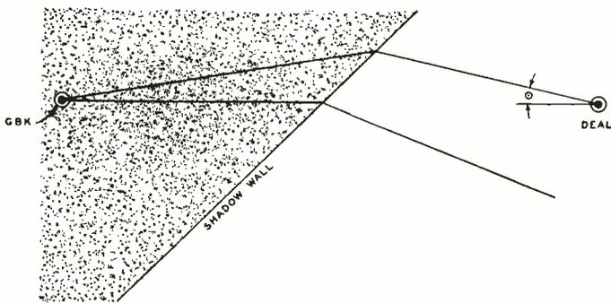
Fig. 3—Suggested way in which the shadow wall affects the receiving angle
