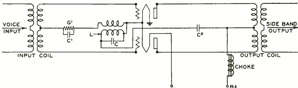
Fig. 2—Modulator circuit of the D-1 System
