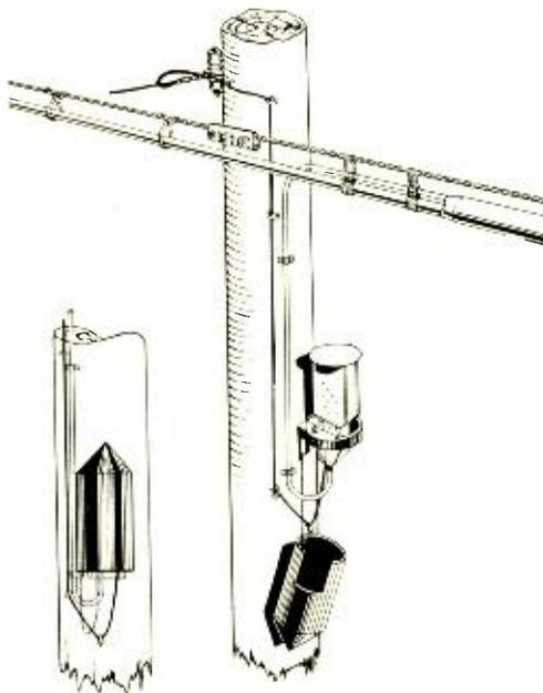
Fig. 3—Method of mounting No. 8 type terminal on telephone pole
