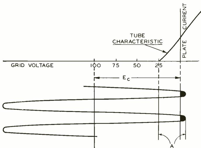
Fig. 3—Production of carrier-frequency oscillations by the oscillator-modulator tubes
