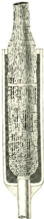
Fig. 2—Diagrammatic sketch showing method of forming pothead
