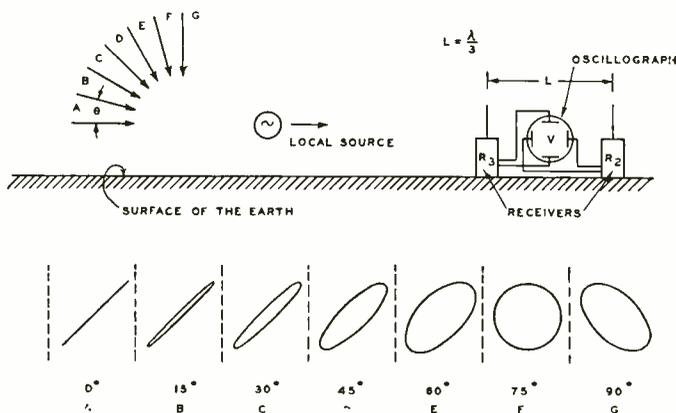
Fig. 2—Arrangement of apparatus for detecting vertical-plane angles
