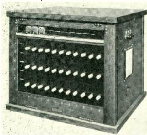
Fig. 1—The 505 P. B. X. uses neither cords nor plugs; all switching is done by manipulating keys mounted on the face of the cabinet
