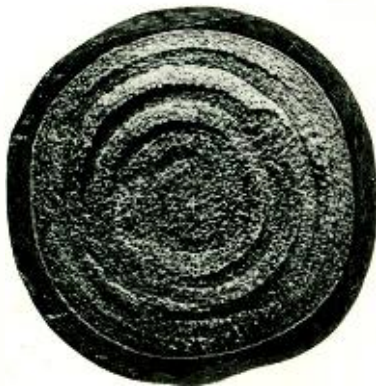
Fig. 2—In this cross-section of the 1200-pair cable also the layered construction is clearly evident
