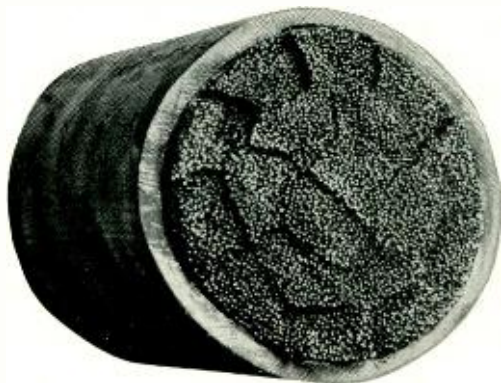
Fig. 3—A cross-section of the 1800-pair cable shows how the eighteen units are formed into the final cable
