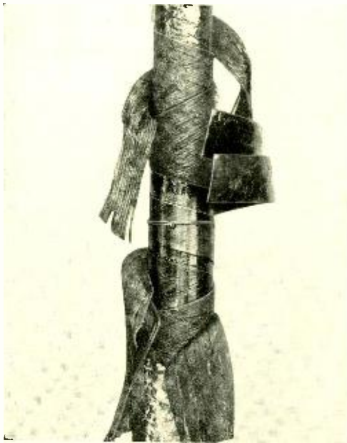
The various layers applied in building up the armoring are here plainly evident
