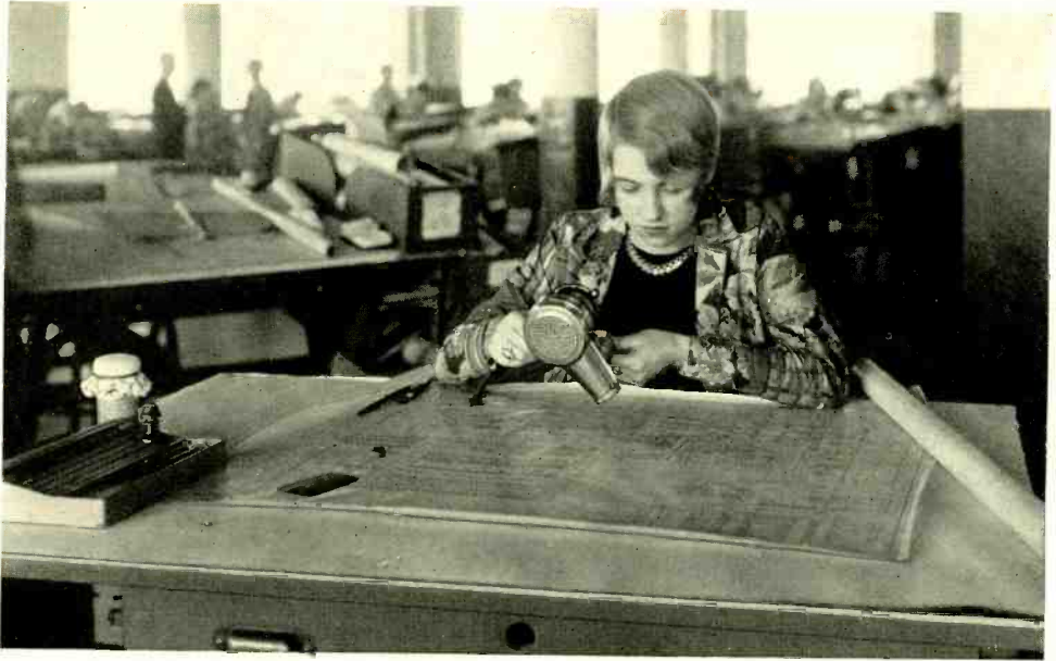
Motor-driven driers reduce the drying time, during which little work can be done on the tracing without danger of blotting
